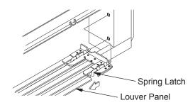
Figure 36 - Removing Louver Panel
